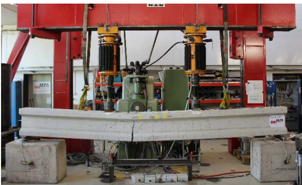
Fig. 3: Fatigue test at iBMB (after failure)
